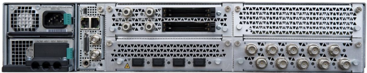
Figure 2. Cisco DCM Series D9902 Rear Panel with AC and DC power supplies, GbE card, ASI card, DRD card, and MFP card
