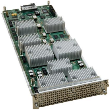
Figure 1. Cisco DCM Series Multi Format Processor Card - Single Layer
