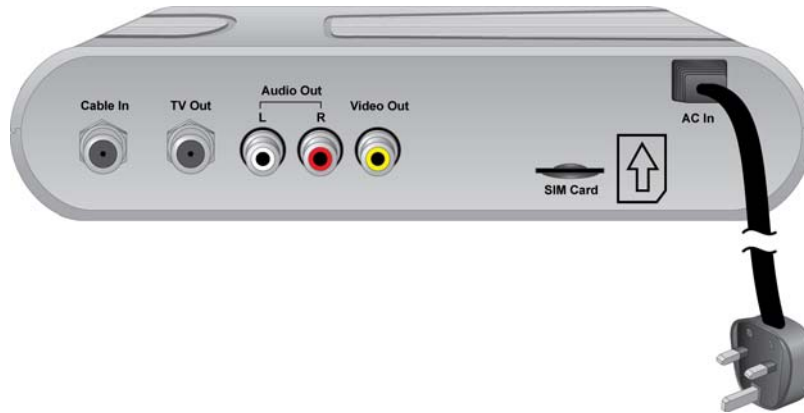
Figure 4. Cisco Z378DVB Back Panel (image may vary from actual product and specification)
